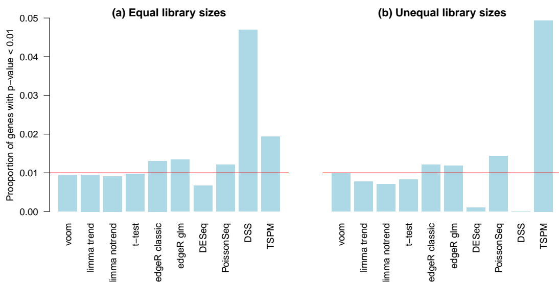
Figure 3: Type I error rates in the absence of true differential expression. The barplots show the proportion of genes with p -value < 0.01 for each method (a) when the library sizes are equal and (b) when the library sizes are unequal. The red line shows the nominal type I error rate of 0.01. Results are averaged over 100 simulations. Methods that control the type I error at or below the nominal level should lie below the red line.
